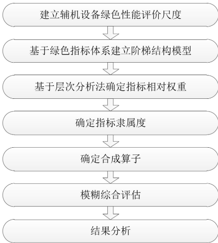
Figure 1. The fuzzy synthetic evaluation method of green grade for engine devices 图 1. 基于模糊层次分析法机舱设备绿色性能评估方法
