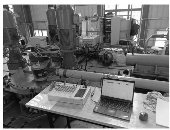
Figure 7. Loading simulation test of the electric steering gear 图 7. 电动舵机加载模式试验
