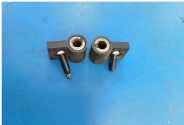
Figure 3. Comparison of positioning component screw fracture
