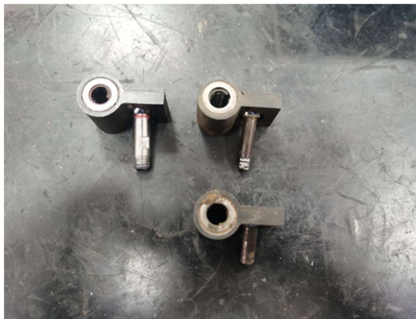
Figure 6. Comparison of screw before and after transformation
