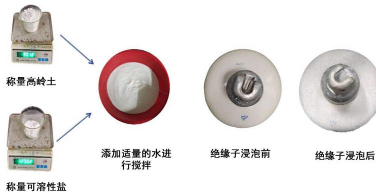
Figure 1. Schematic diagram of the artificial contamination process of insulators 图 1. 人工污秽绝缘子染污过程示意图
