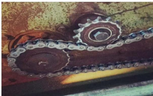
**Figure 1.** On-Site actual picture of the original storage cabinet horizontal carriage conveyor belt transmission tensing device
