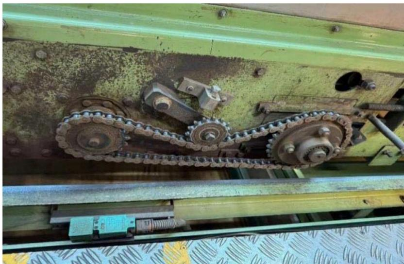
Figure 16. Installation site photo of the improved storage cabinet horizontal carriage conveyor belt transmission chain tensioning device
