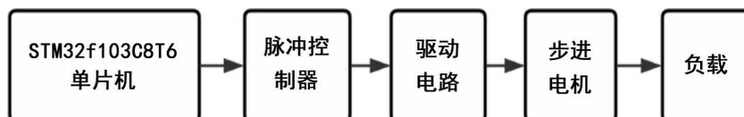
Figure 3. Block diagram of the stepper motor control system
