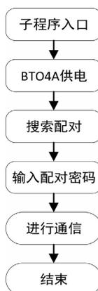
Figure 7. Flowchart of the BT04-A bluetooth module program
