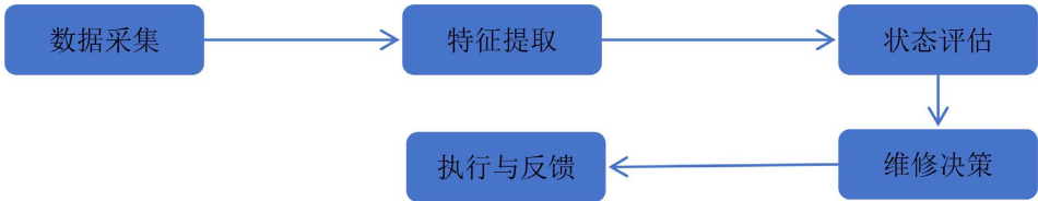
Figure 1. Flowchart of predictive maintenance implementation for cigarette packaging machines 图 1. 卷烟包装机预测性维护实施流程图
