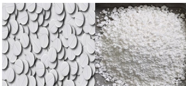
Figure 2. Samples of tablet-shaped and irregular-shaped LiOH particles 图 2. 药片状和不规则片状 LiOH 颗粒样品图
