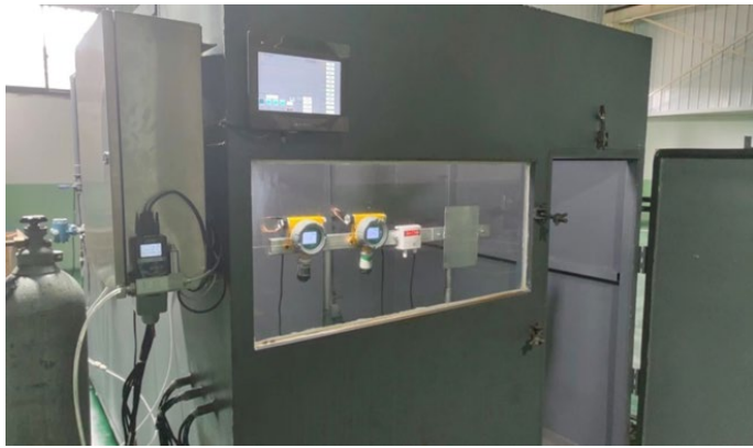
Figure 7. Environmental simulation test chamber (volume: 4.1 m 3 ) 图 7. 环境模拟试验舱(体积：4.1 m 3 )
