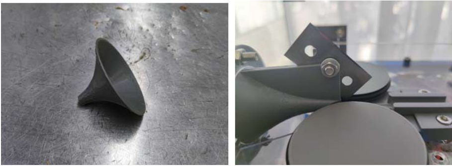
Figure 2. Schematic diagram of the trumpet-shaped inlet (left) and cutting blade (right) 图 2. 喇叭状入口(左)与切割刀片(右)示意图
