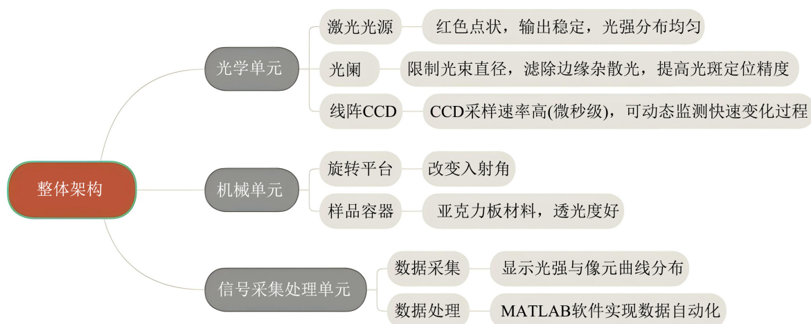
Figure 4. Schematic of experimental system structure 图 4. 实验系统结构图
