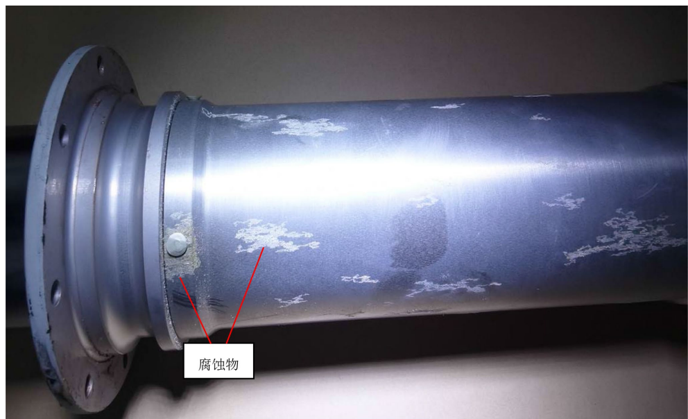
Figure 1. Corrosion of structural components 图 1. 结构件腐蚀
