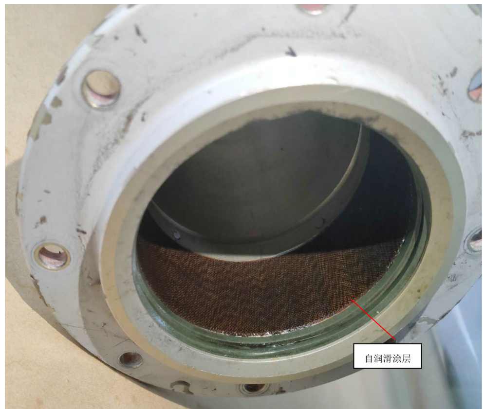
Figure 2. Self-lubricating coating inside the upper and lower support ring assemblies 图 2. 上下支撑环组件内的自润滑涂层
