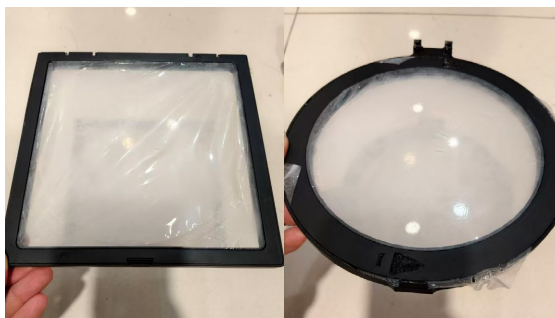
Figure 11. Comparison of square frame and ring frame PE film spreading 图 11. 方形框与环形框 PE 膜展平对比
