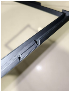
Figure 9. Clip structure printed flat on ABS material 图 9. ABS 材料平放打印的卡扣结构
