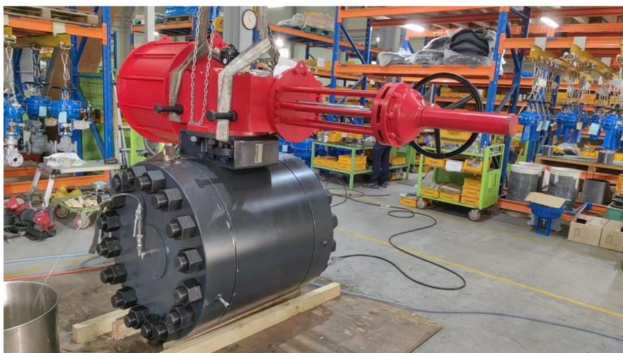
**Figure 7.** Test on the shell and sealing of the triple-eccentric butterfly valve
