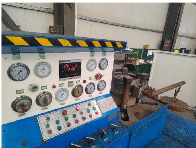
**Figure 8.** Opening and closing torque test of triple-eccentric butterfly valve
