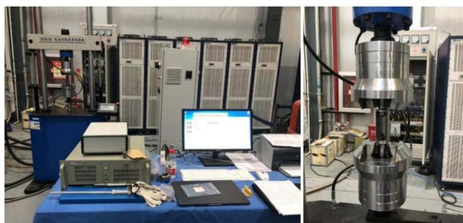
Figure 2. Servo fatigue tester (Left) and damping pad vibration tools (Right)
