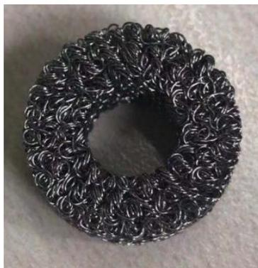
Figure 1. Metal rubber specimen
