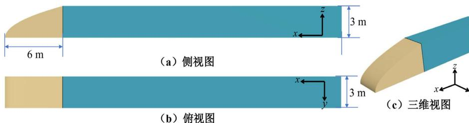
Figure 7. Train geometry and dimensions in Japanese dynamic models
