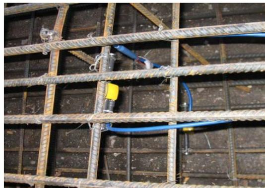
Figure 7. Pre embedded strain gauge
