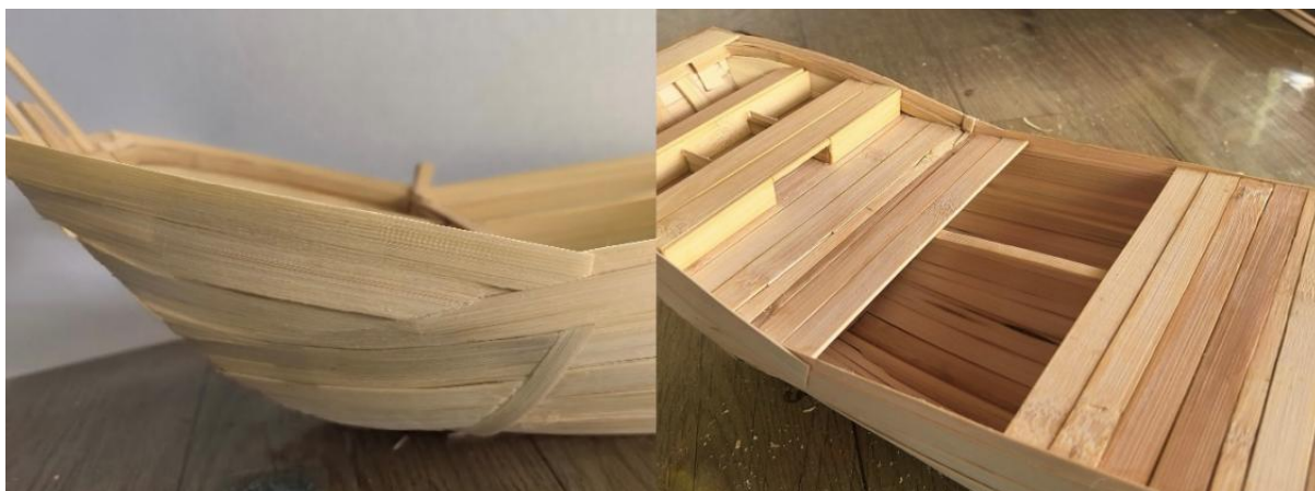
Figure 11. Bow skinning and deck splicing sealing 图 11. 船头蒙皮与甲板拼装封口
