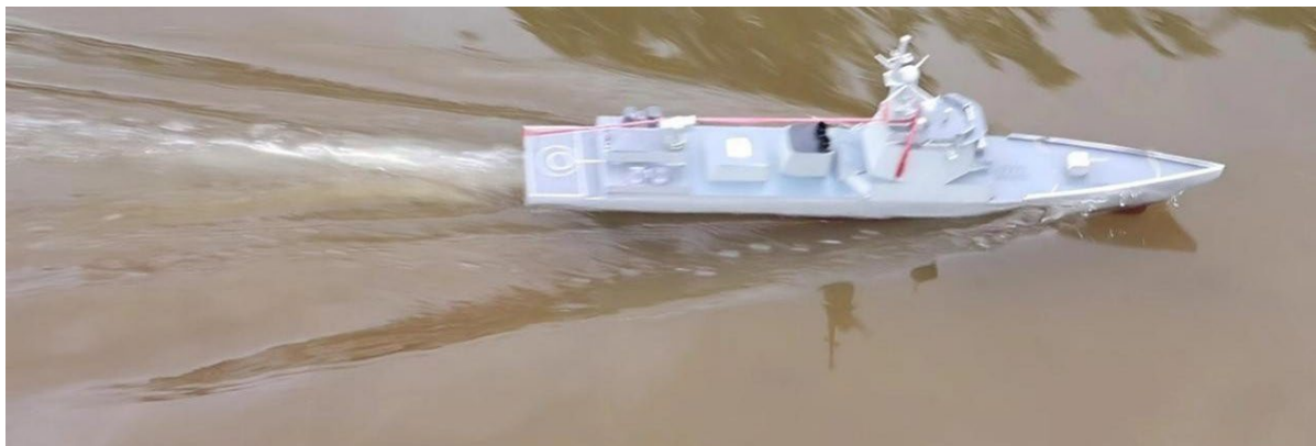
Figure 20. Wave-making of vessel in experiment 图 20. 舰船试验航行兴波
