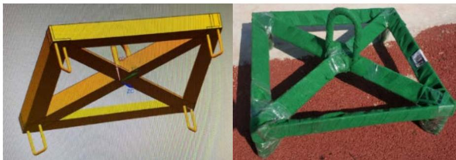
Figure 19. 3D model and physical photos of antenna reflector lifting fixture
