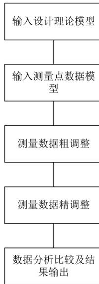
Figure 7. Flowchart for freeform surface profile analysis
