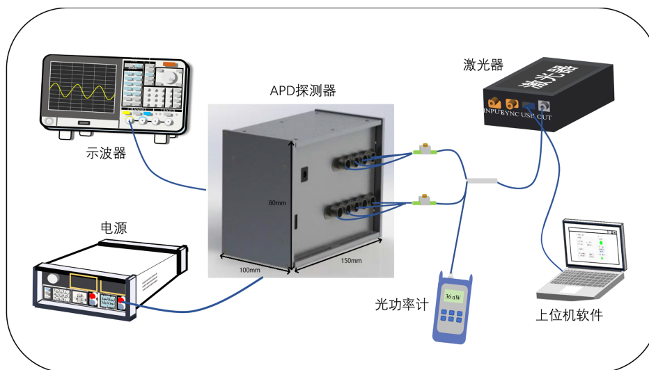
Figure 8. Detector responsivity test experimental setup diagram
