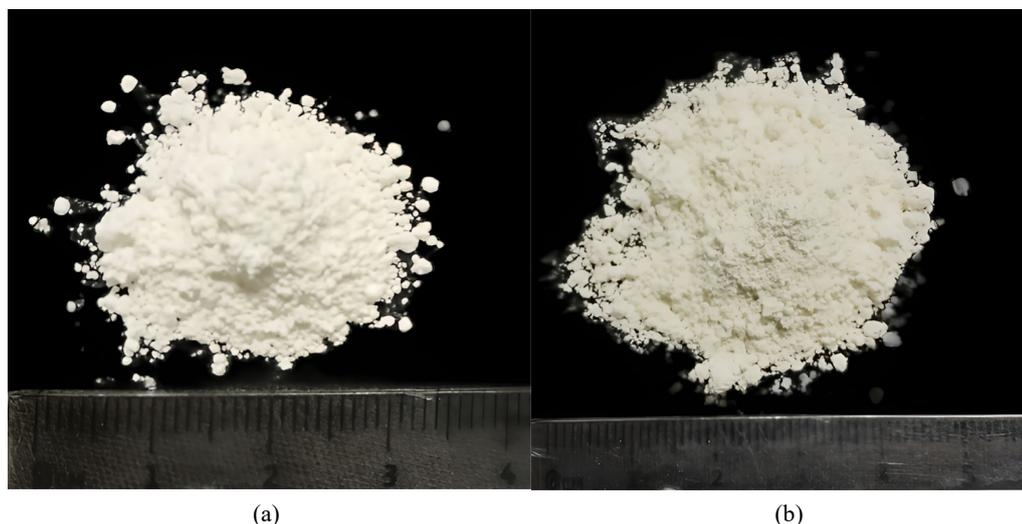
**Figure 2.** Powder diagrams: (a) Pearl powder; (b) Shell powder
