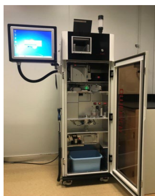
Figure 2. Cigarette physical property comprehensive testing system 图 2. 烟支物性综合测试系统
