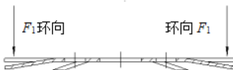
Figure 2. Spring washer and its force diagram
