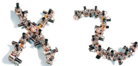
Figure 7. The PolyBot chain reconfiguration system
