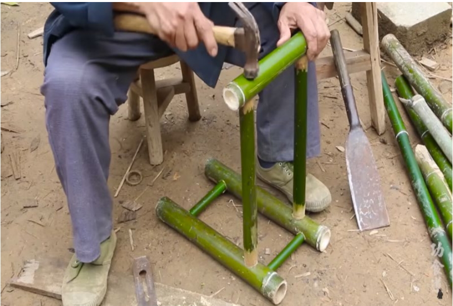
Figure 1. Connection of bamboo joints 图 1. 竹节的连接 1
