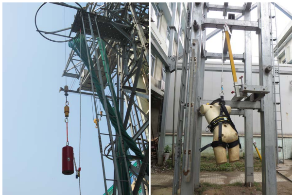
Figure 18. Impact test of rope type fall arrester and insulation ladder 图 18. 绳索式防坠器及绝缘梯台冲击试验
