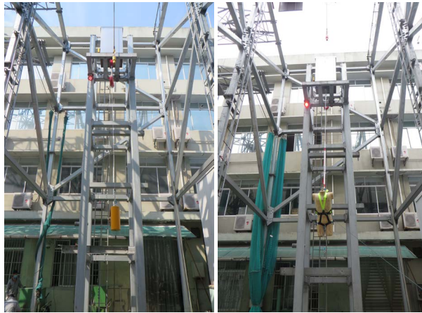
Figure 17. Seat belt and speed difference impact test 图 17. 安全带及速差器冲击试验
