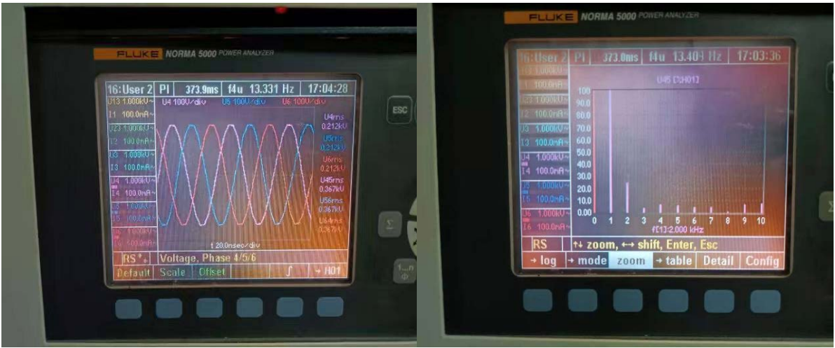
Figure 10. Back electromotive force waveform and harmonic decomposition diagram 图 10. 反电动势波形及谐波分解图
