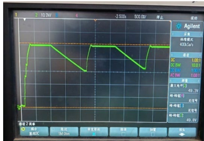
Figure 9. Voltage waveform during repeated startup with a 10,000 \mu\text{F} capacitive load 图 9. 带 10,000 \mu\text{F} 容性负载后重复启动时电压波形
