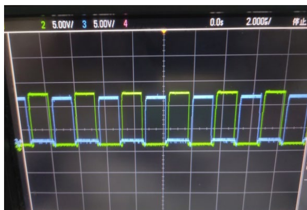
Figure 6. Gate waveforms of V2 and V3
