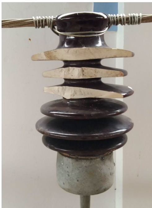
Figure 2. Training set of damaged insulators 图 2. 训练集破损绝缘子
