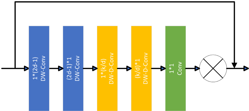
Figure 4. LSKA series decomposition diagram 图 4. LSKA 串联分解示意图
