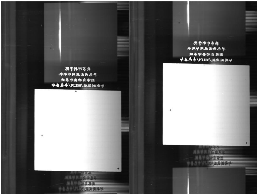
Figure 5. Reference image of the first color plate (left) and the image to be aligned (right) 图 5. 第一色板基准图像(左)与待套准图像(右)
