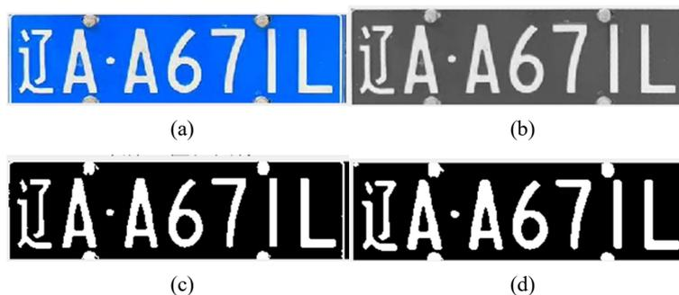
**Figure 15.** (a) Precisely located license plate; (b) Grayscale conversion; (c) Binarization; (d) Morphological operation
