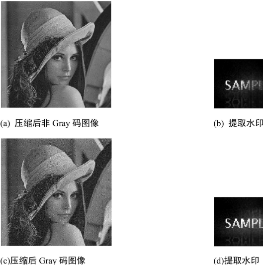
Figure 4. Comparison of watermark extraction using gray code vs non-gray code after compression 图 4. 压缩后 Gray 码与非 Gray 码水印提取对比
