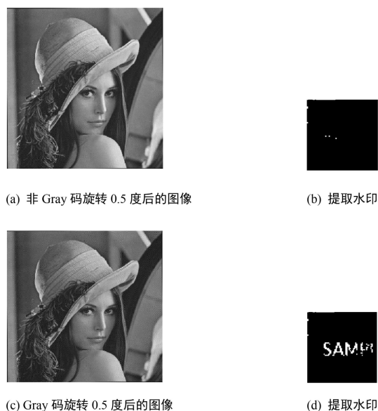
Figure 6. Comparison of watermark extraction using gray code vs non-gray code after rotation 图 6. 旋转后 Gray 码与非 Gray 码水印提取对比
