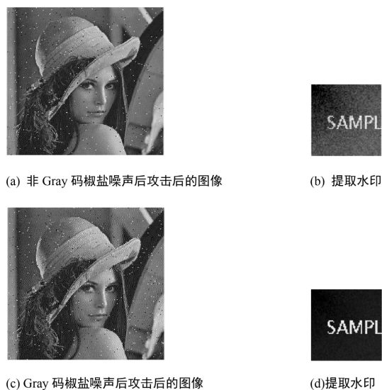
Figure 8. Comparison of watermark extraction using gray code vs non-gray code under salt-and-pepper noise 图 8. 椒盐噪声后 Gray 码与非 Gray 码水印提取对比
