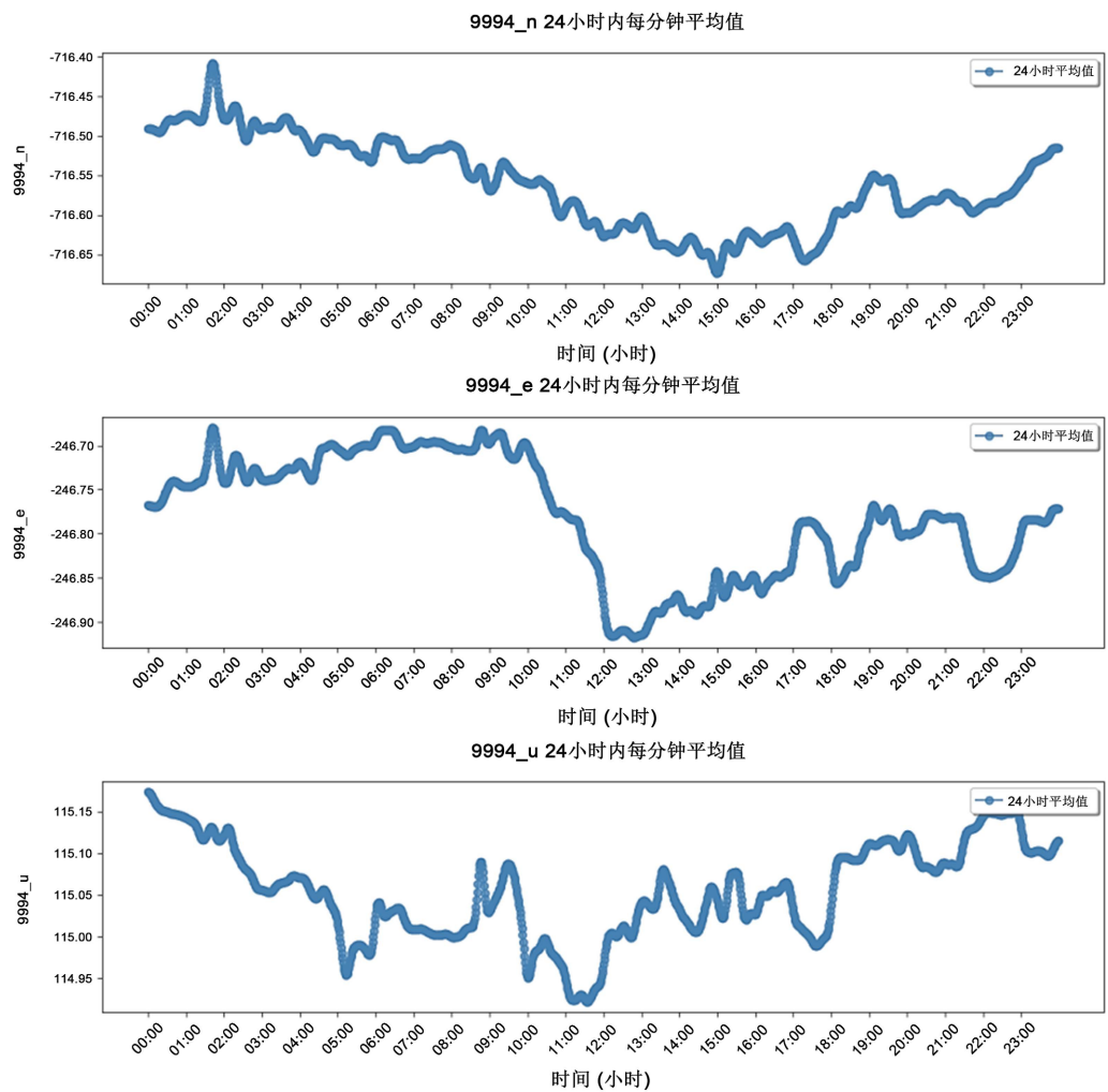
Figure 6. Intraday average coordinate variation of the mid-span measurement points of the bridge (Unit: m) 图 6. 大桥跨中测点位日内平均坐标变化(单位: m)
