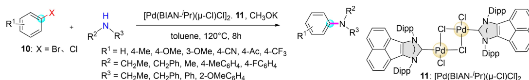
Figure 10. Structure of complex 11 and catalytic Buchwald-Hartwig coupling reaction
