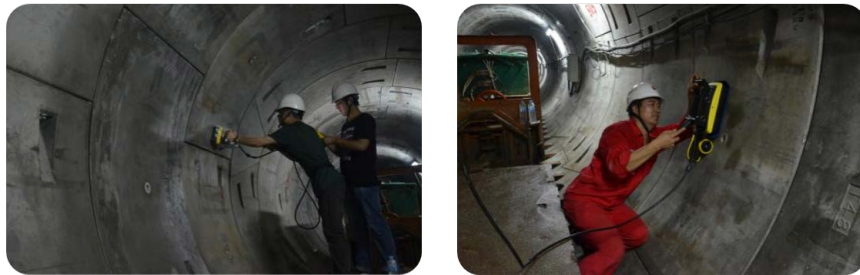
Figure 2. The inspection of segment back filling grouting effect using geological radar
