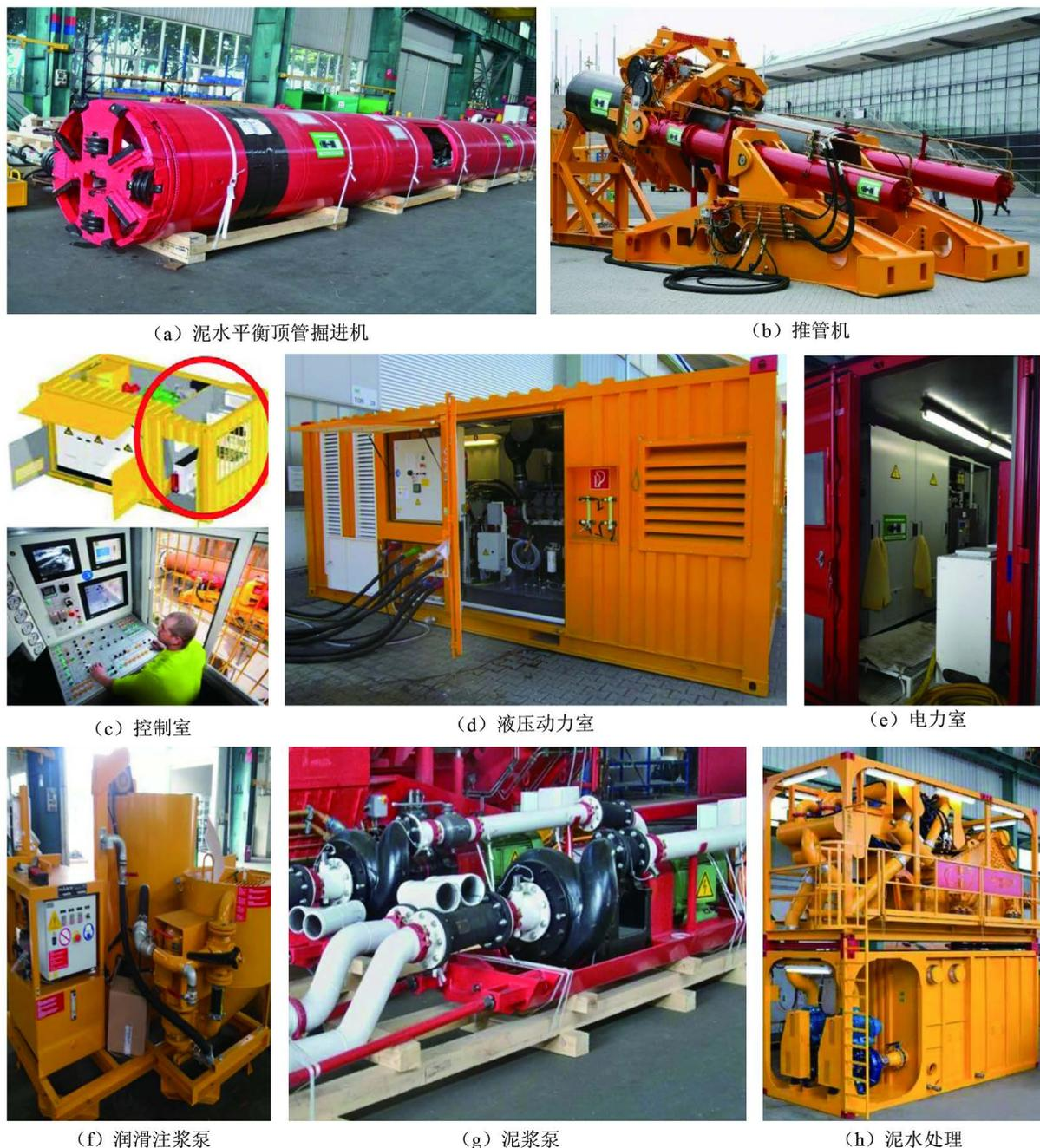
Figure 1. The major equipment used in construction
