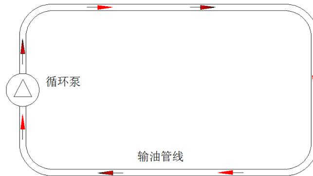
**Figure 3.** Schematic diagram of the lipophilic test device for the inner wall of the tubing
