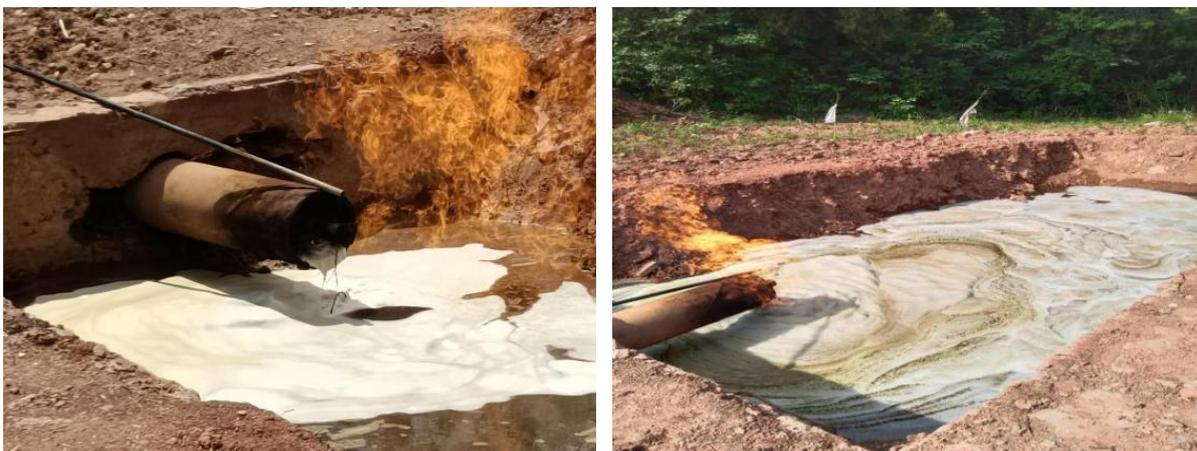
**Figure 3.** Blowout at the third stage of well M-AH29 plugging removal
