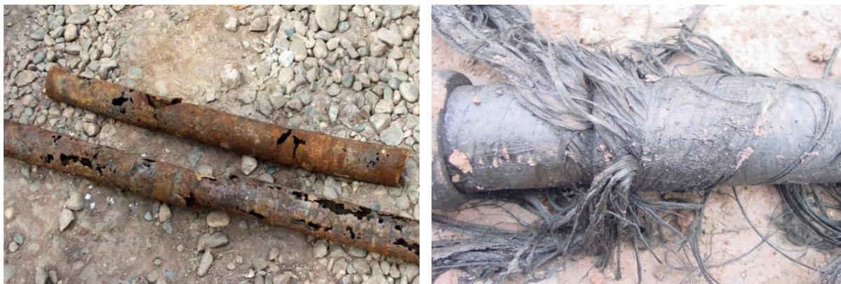
**Figure 1.** Downhole tubing corrosion and FRP coating falling off
