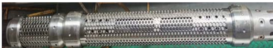
Figure 2. Metal mesh protective sleeve of new dipole acoustic logging tool
