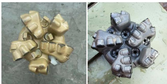
**Figure 5.** Before and after photos of the triple-opening 152.4 mm MDS1516 bit in Jing11-78H1 well
