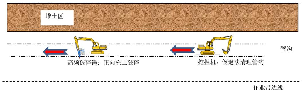
**Figure 5.** Schematic diagram of equipment positioning and construction direction
