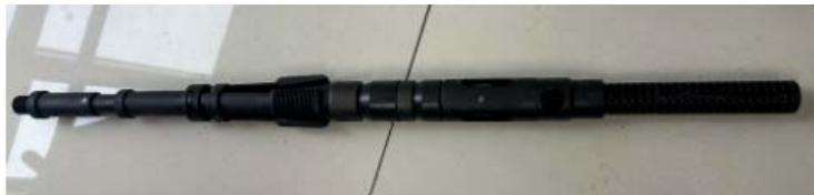
Figure 9. Drop downhole throttle of Jinqian12-6-H1
