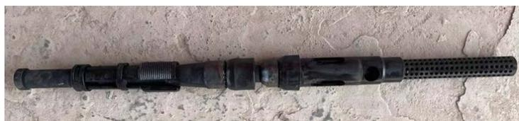
Figure 10. Remove downhole throttle of Jinqian12-6-H1
