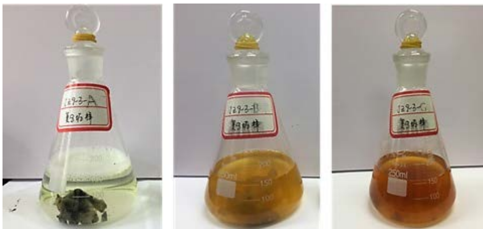
Figure 5. Scale dissolution experiment 图 5. 垢样溶解实验
