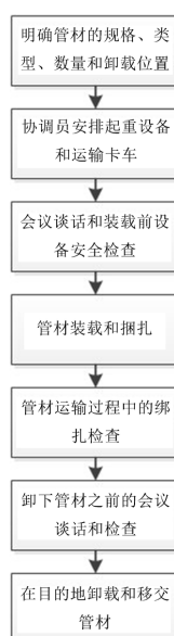
Figure 1. Pipe transport flow chart
