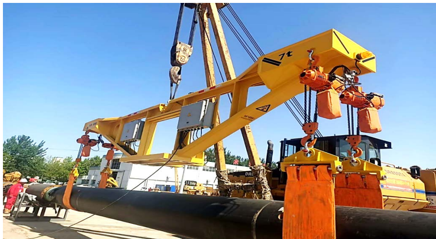
Figure 1. Electric drive pipe handling equipment 图 1. 电驱动转管吊具
