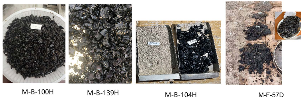
Figure 1. Map of bitumen cuttings encountered by drilling in M oilfield development well 图 1. M 油田开发井钻遇储层沥青岩屑图
