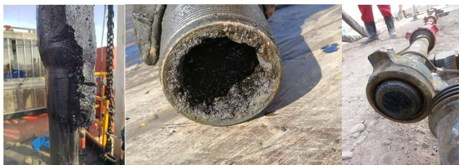
Figure 1. Asphalt deposition found in production tubing and well flowlines
