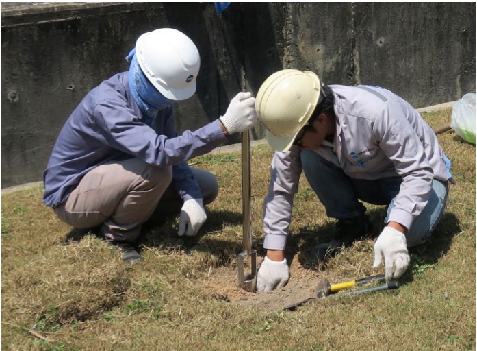
Figure 8. Soil sampling 图 8. 土壤取样
