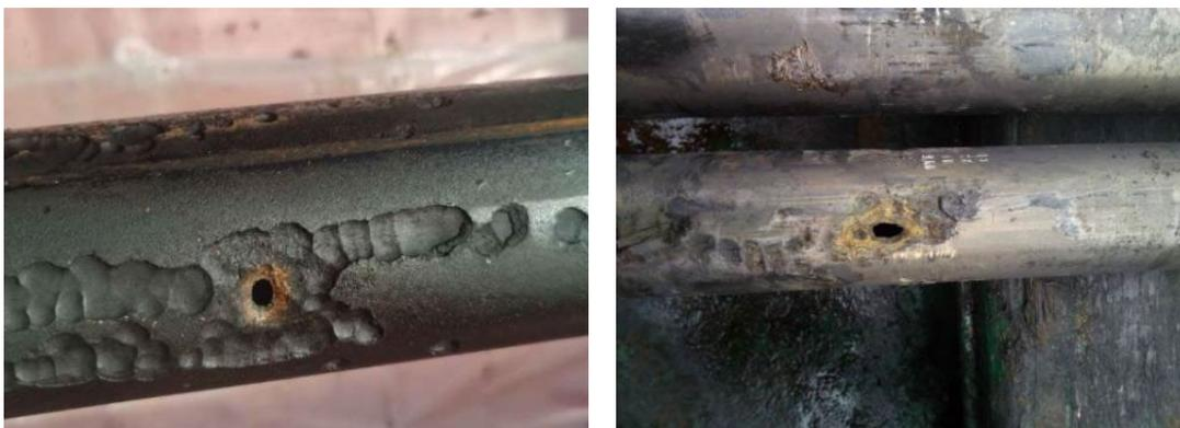
**Figure 1.** Corrosion perforation of tubing caused by acidification
